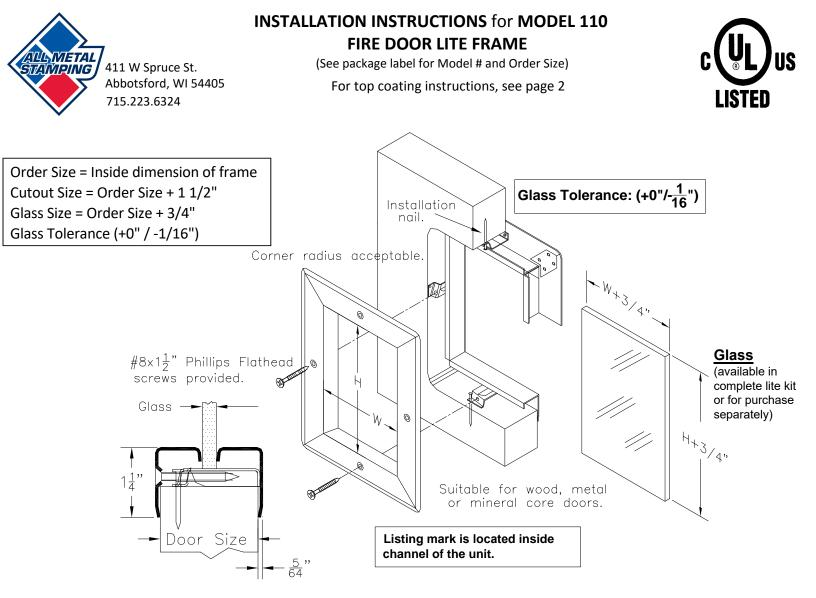
**NOTE ON GLAZING TAPE:** Some types of glass & some very large frames require glazing tape. Scan the QR Code (right) or visit *www.allmetalstamping.com* for a listing of approved glazing, fire ratings, or additional installation requirements such as tape or intumescent.
